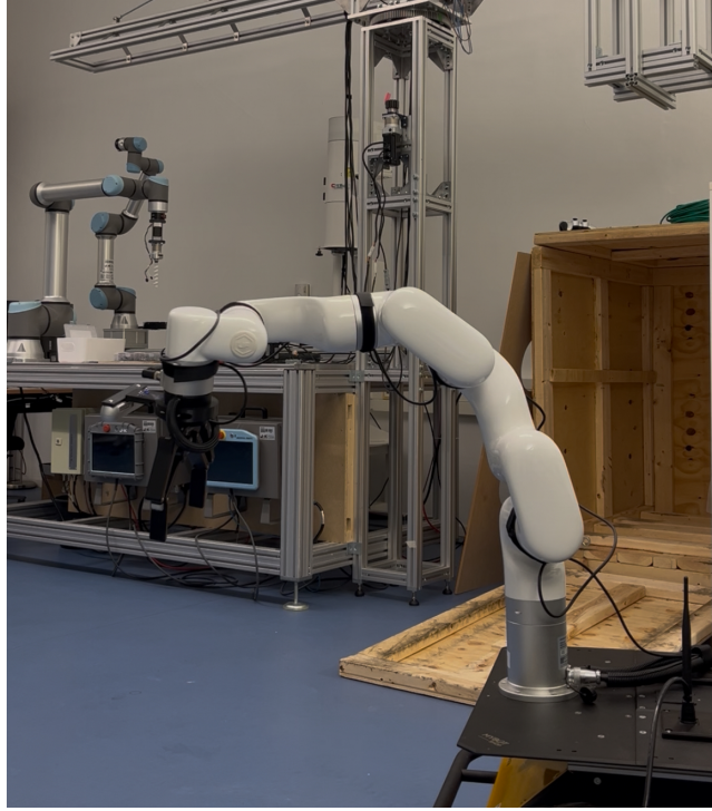
Figure 5.1 Real-world experimental setup showing the physical Clearpath Husky A200 mobile manipulator platform with the UFactory xArm6 manipulator during planning experiments.
